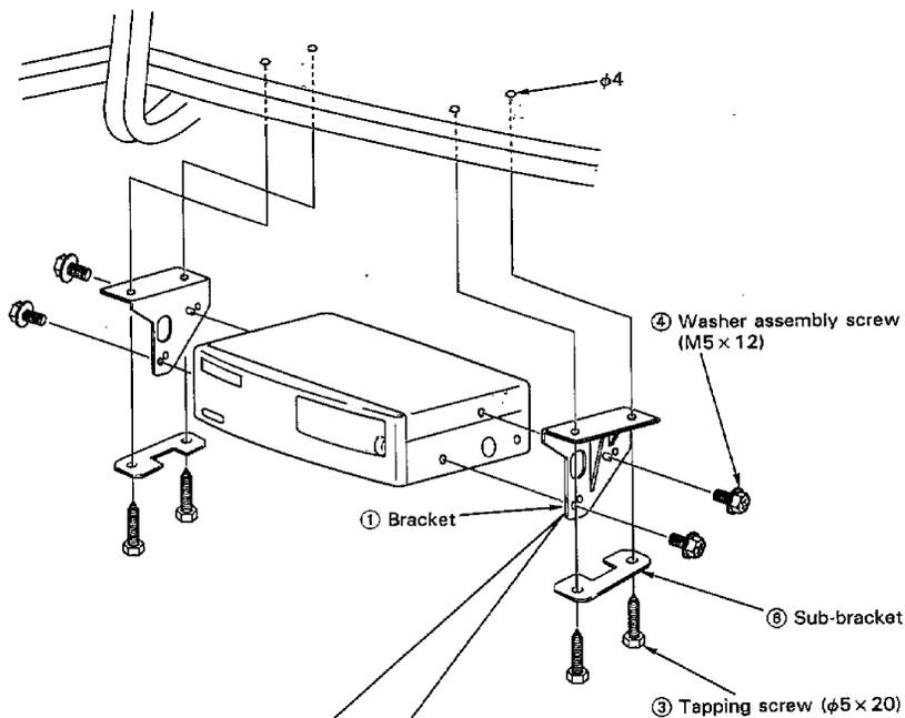
Attach the brackets with the screws inserted in the blackened holes. (Do the same for the left side also.)
