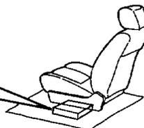
Install the RF modulator unit beneath the front seat using Metal fixture and Bind head screw as shown in the above figure.
