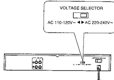
Move switch lever to match your line voltage with a small screwdriver or other pointed tool.
