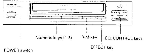
**1** Press the POWER switch of this unit to ON.
