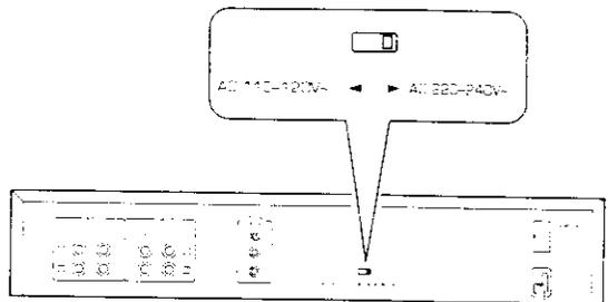
Move switch lever to match your line voltage with a small screwdriver or other pointed tool.
