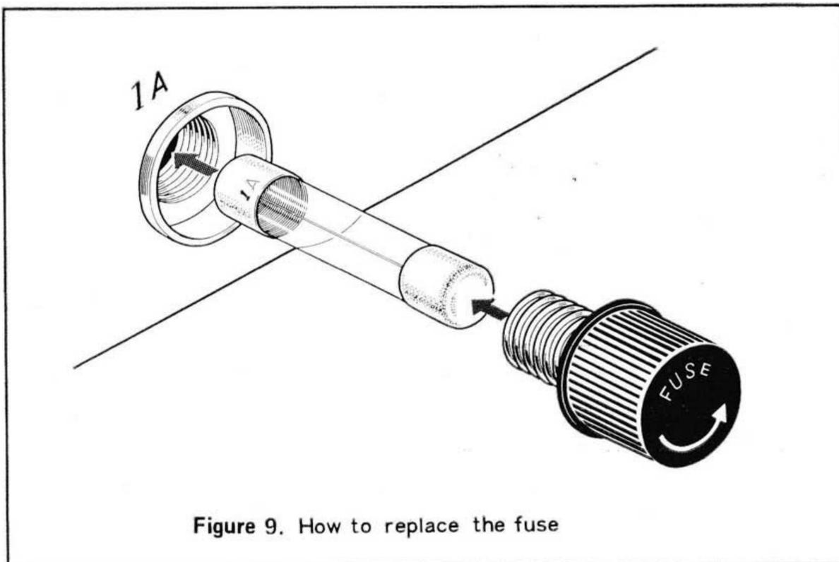
Figure 9. How to replace the fuse
