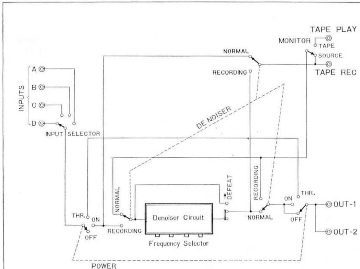
Figure 5 KF-8011 Function Diagram
