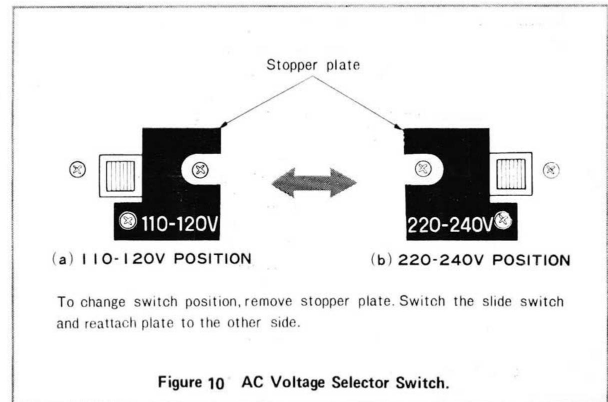
Figure 10 AC Voltage Selector Switch.
