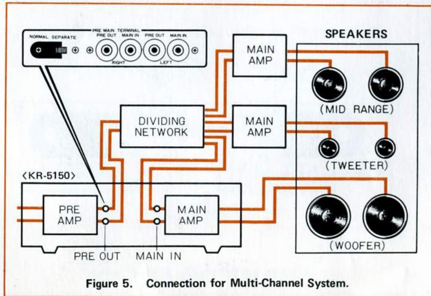
Figure 5. Connection for Multi-Channel System.
