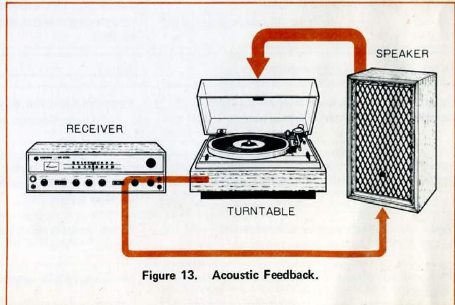
Figure 13. Acoustic Feedback.
