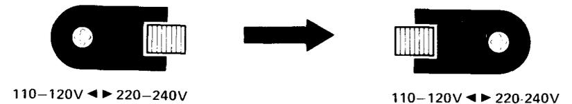
Figure 8. AC Voltage Selector Switch.
