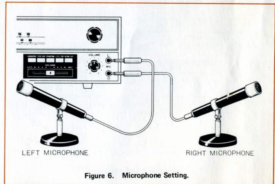
Figure 6. Microphone Setting.
