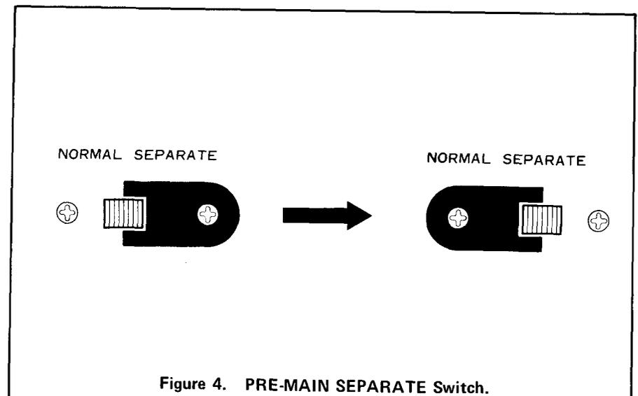
Figure 4. PRE-MAIN SEPARATE Switch.
