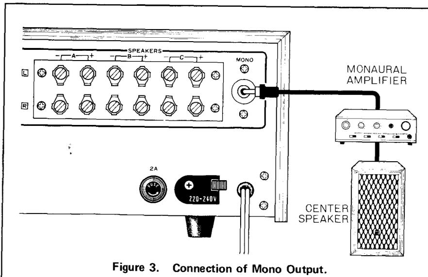
Figure 3. Connection of Mono Output.
