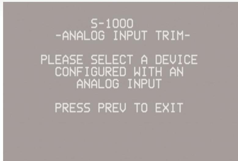
To select an analog device, first exit the menu program by pressing the menu key (29). Then press the analog device key [for example, the tape key (14)] on the remote control. The front panel displays the device selection. Enter the menu program and follow the procedure for selecting analog input trim described on the next page.
