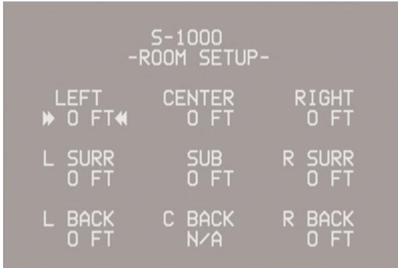
When you access the **ROOM SETUP** screen, the cursor is blinking at the **LEFT** loudspeaker. Use the direction and enter keys to navigate the screen, select loudspeakers, and enter the correct distance (0 to 30 feet) from the main listen position to the loudspeaker.
