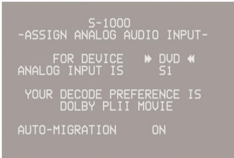
Use the direction and enter keys to scroll through and select the device you want to configure, select the MIGRATION/REC input, and choose the analog mode, if mode options are available.
