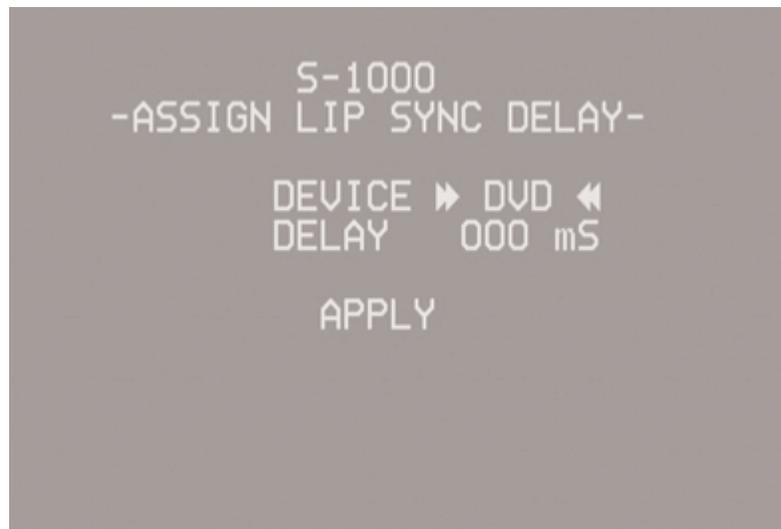
Use the direction and enter keys to scroll through and select the device you want to configure for lip synchronization. Make sure that the device is already configured for the digital audio source and display you intend to synchronize. Power on the source and display, and start playing a program.
