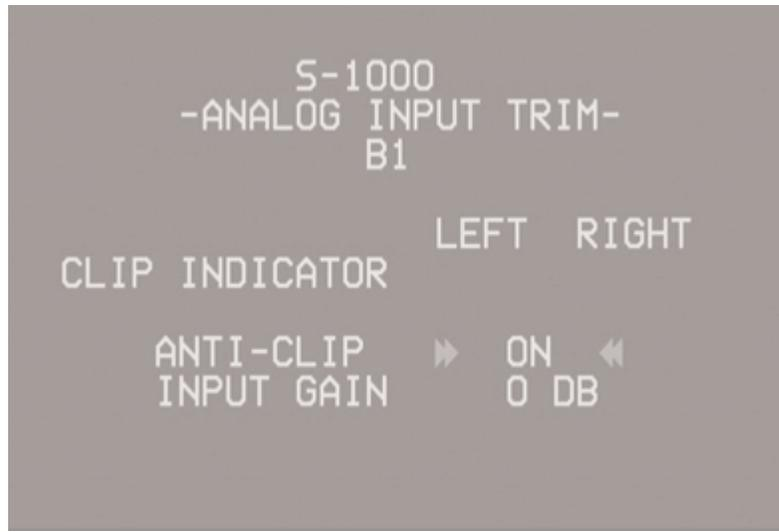
Use the direction keys (75) to select the anti-clip option you want (ON or OFF) and the input gain decibel level. Krell recommends leaving anti-clip ON.
