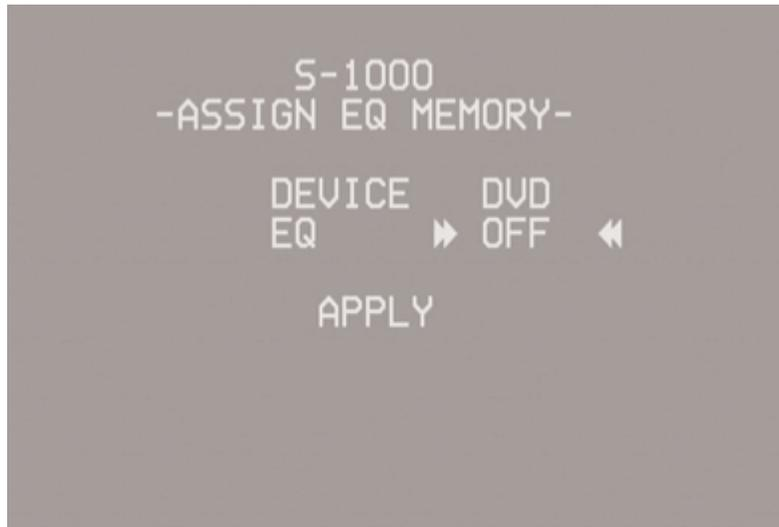
Use the direction and enter keys to scroll through and select the device to which you want to assign EQ memory. Select EQ memory 1,2,3,or 4 or select OFF.
