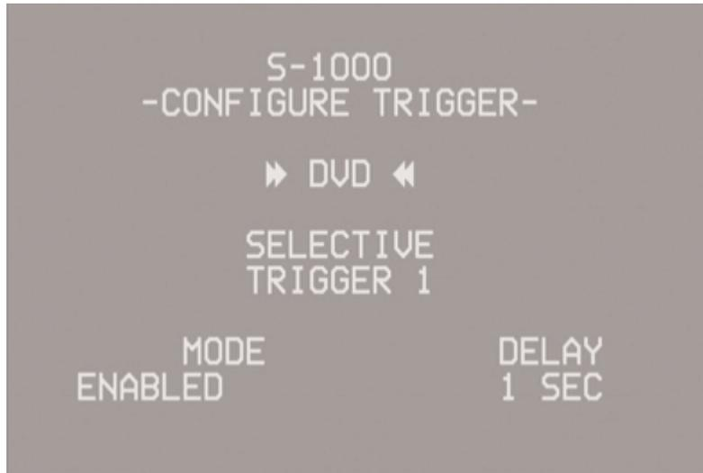
Use the direction and enter keys to select the source device. Select ALL TRIGGERS to configure all triggers at once, or choose SELECTIVE to configure triggers individually. The delay is only available when a trigger is set to ENABLED. There is a three second delay after you select ENABLED, before the trigger turns on. The trigger turns off immediately when you select DISABLED.
