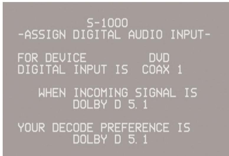
Use the direction and enter keys to scroll through and select the digital device you want to configure, select the digital input, and choose the default mode for the four major surround sound digital formats: DOLBY DIGITAL 2.0, DOLBY DIGITAL 5.1, DTS 5.1, and PCM. You can choose a decoding preference for each of these signals under YOUR DECODE PREFERENCE IS. *For more information, see **Decoding Modes for the S-1000**, on page 60.*
