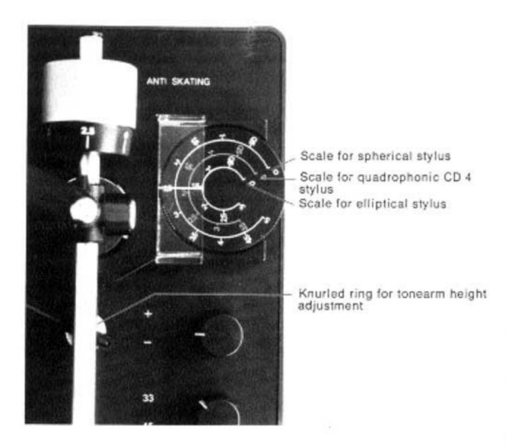
Using a JVC 4 MD-20X Shibata Quadrophonic stylus, with an optimum pressure weight of 1.7 grams, set the number at 1.7 on the 'A' scale.
