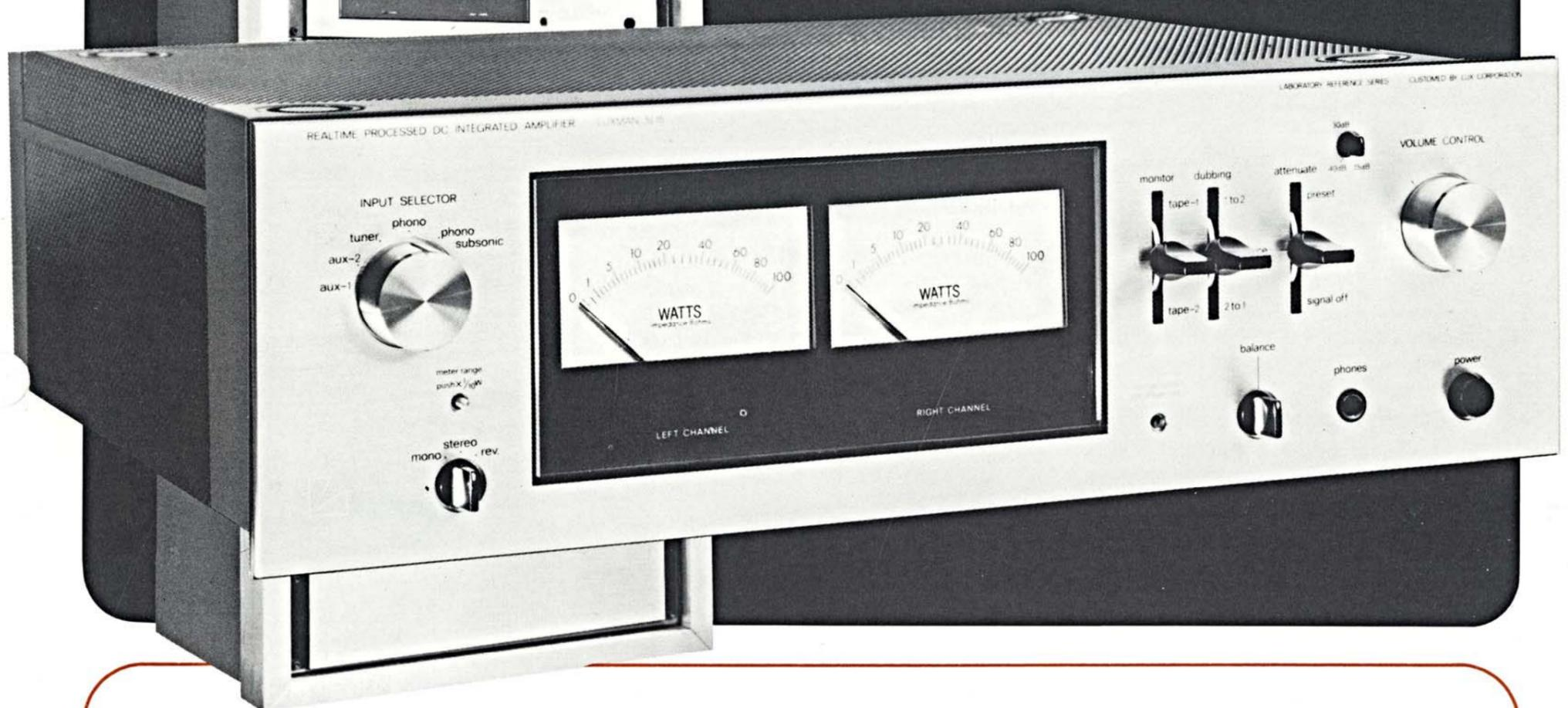
The Luxman 5L15 integrated amplifier is rated at 80 watts/channel minimum continuous power, both channels driven into 8 ohms from 20 Hz to 20 kHz, with no more than 0.02% total harmonic distortion. Intermodulation distortion is also a low 0.02% at rated output. Both the preamplifier and power amplifier sections are direct-coupled DC design, for high phase linearity, low transient intermodulation distortion and extremely wide-band response.
