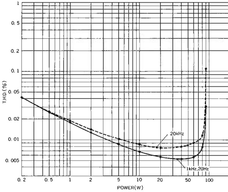
L-55A EQ. AMP OUTPUT LEVEL VS T.H.D. (INPUT:PHONO-I, OUTPUT:REC. OUT, 400Hz HIGHPASS FILTER ON FOR 1kHz & 20kHz)
