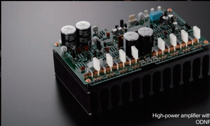
High-power amplifier with 4-parallel module, ODNF circuit, version 4.0
