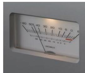
Needle-type meter with electric bulb-colored illumination
