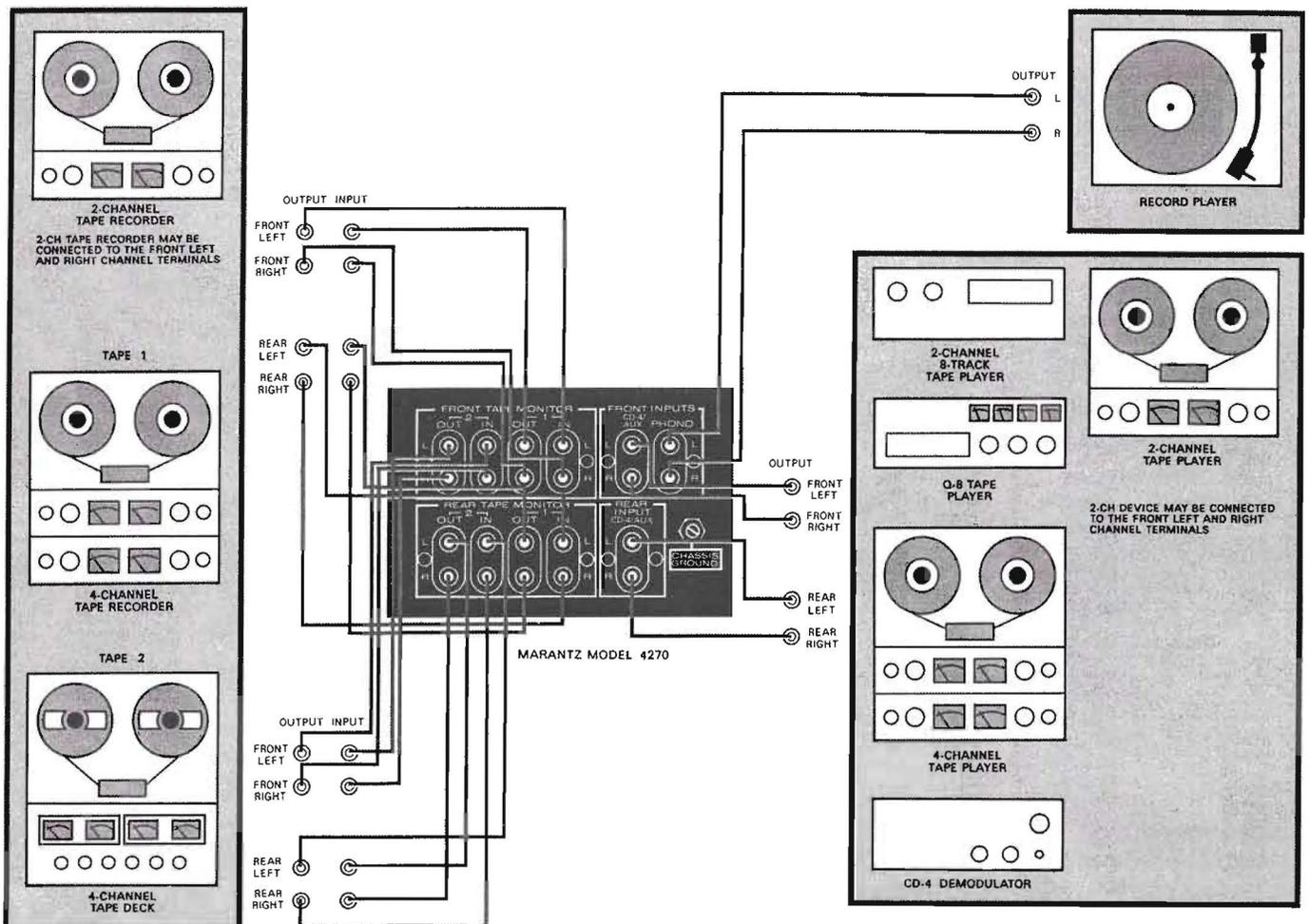
Figure 3. Connection Diagram
