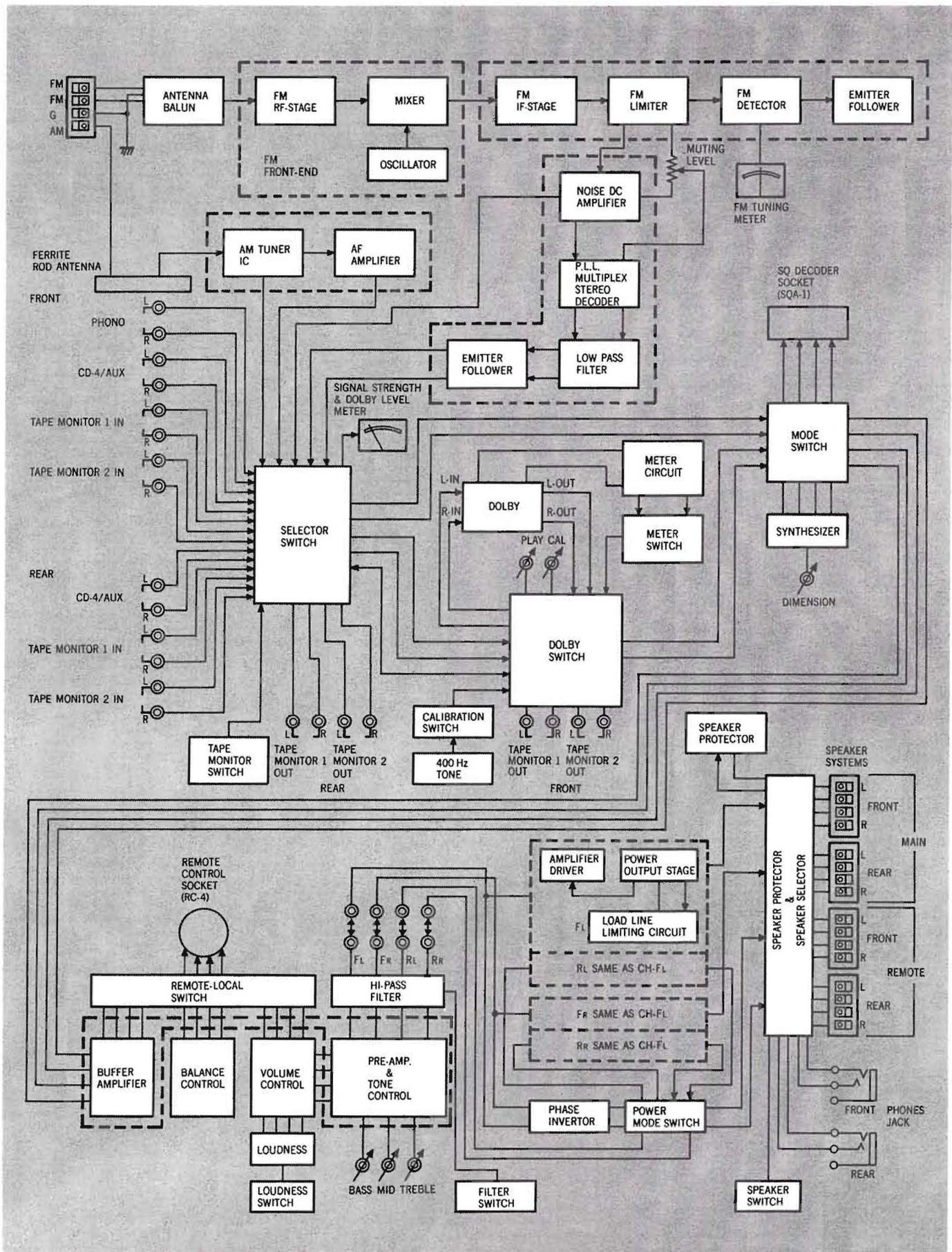
Figure 14. Block Diagram
