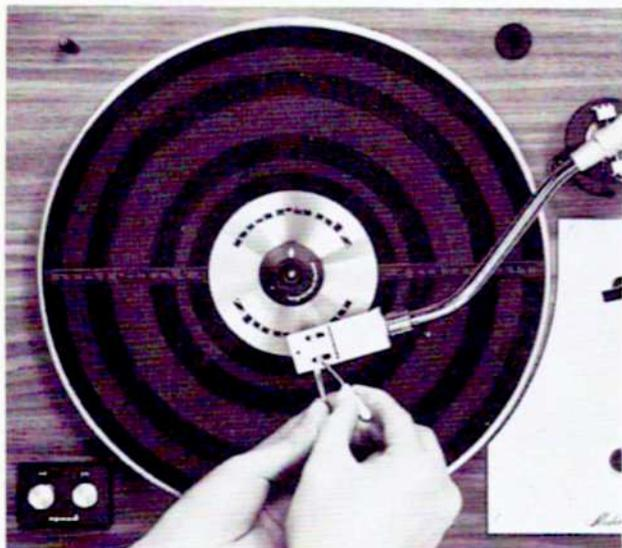
Figure 4. Stylus Overhang Adjustment
