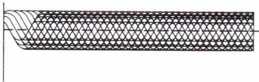
Position of the oscilloscope: 0,5 µs/div. Amplitude about 1,5 Vpp.
