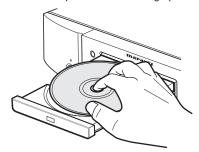
In the case of a single (8 cm) CD, align it with the indentation in the center of the tray.
