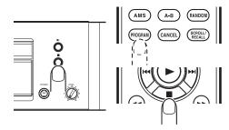
The PROG indicator stops flashing and lights up instead, and the program is entered.
