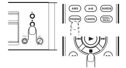
The PROG indicator in the display stops flashing and lights up instead, and the delete program is entered. Up to 30 tracks can be deleted from the program.
