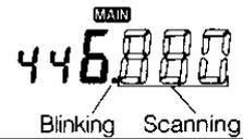
**4** Hold down the **[F]** key and press the **[SCN.P.S]** key. (The All Scan is started.)
