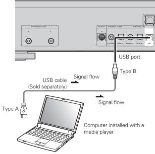
Plug that fits the shape of the connection device connector
