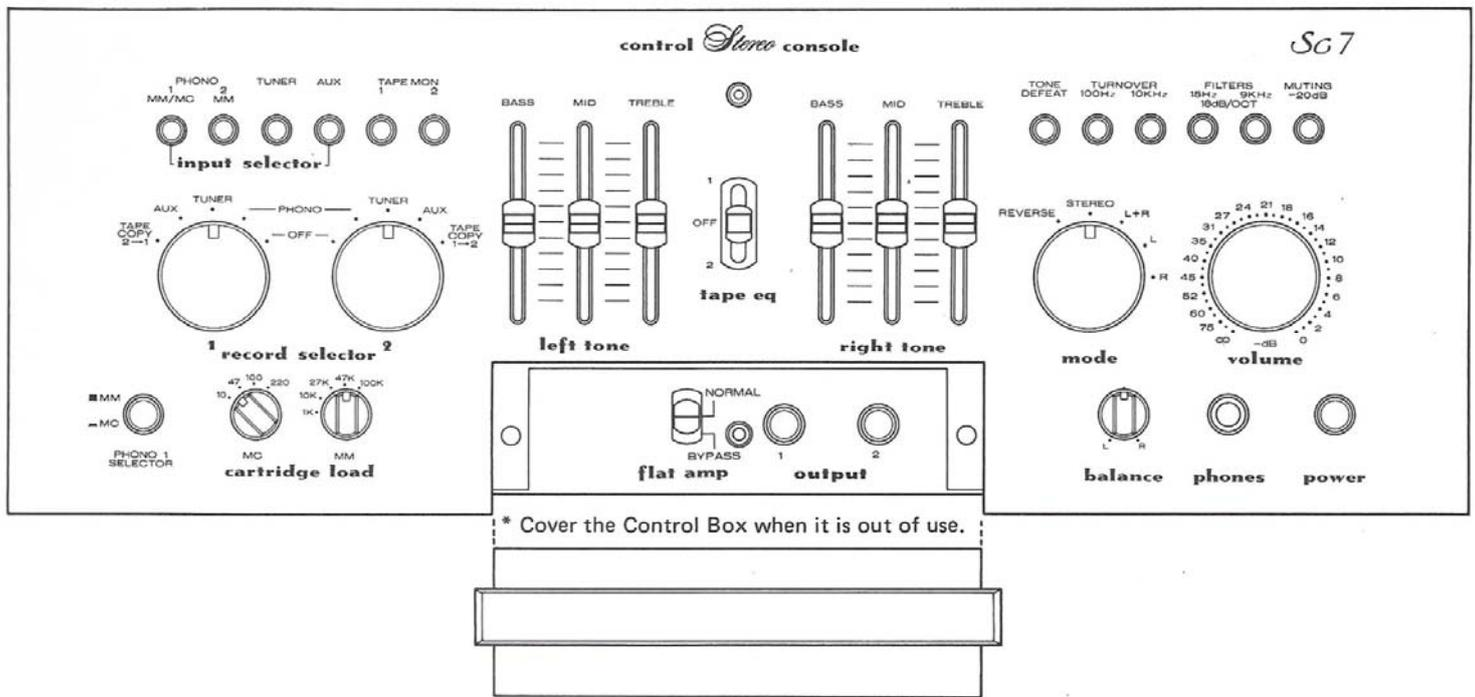
Figure 3. Front Panel Controls and Features
