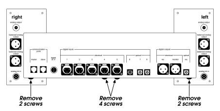
3. Carefully slide the top cover toward the rear of the unit and remove it.
