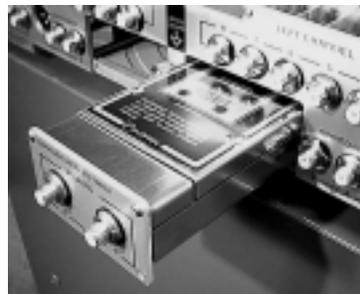
**Do not force!** The phono preamp modules should slide in easily. If a phono preamp module does not slide in easily, remove it and repeat step 7.
