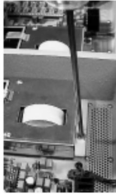
**11. Carefully lift connector ends of cables out of holes in phono preamp top cover.**
