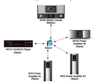
The figure below illustrates a typical ML Net setup:
