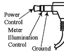
1/8 inch stereo mini phone plug is used for connection to the Power Control, Trigger and Pass-Thru Outputs on the C50.
