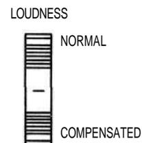
This switch converts the VOLUME control to a loudness compensated control when in the COMPENSATED position.
