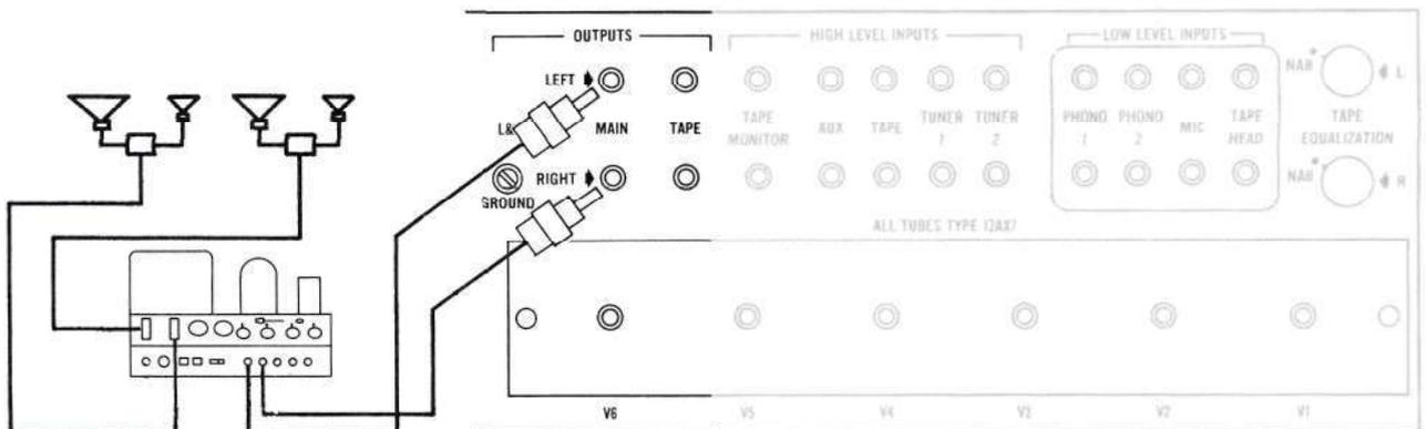
Figure 9. MAIN Output Connected to Power Amplifiers
