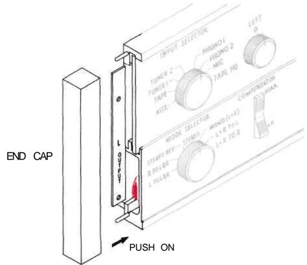
Figure 5. Fitting of Panel End Caps to Panel
