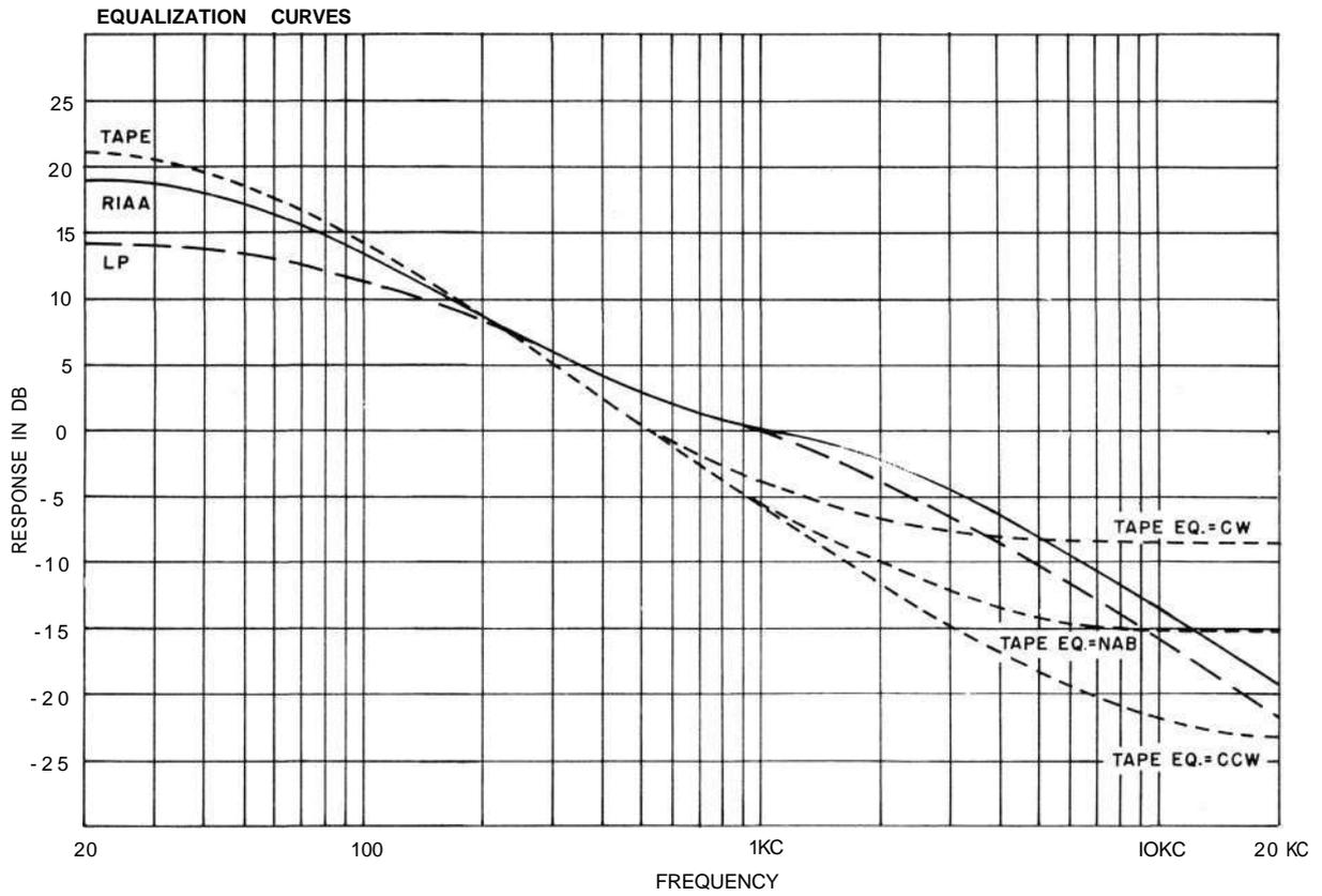
Figure 10. Equalization curves.
