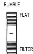
Low-frequency rumble noise below 50cps created by a turntable or record changer and acoustically coupled feedback are reduced when the RUMBLE filter button is pushed to the FILTER position.
