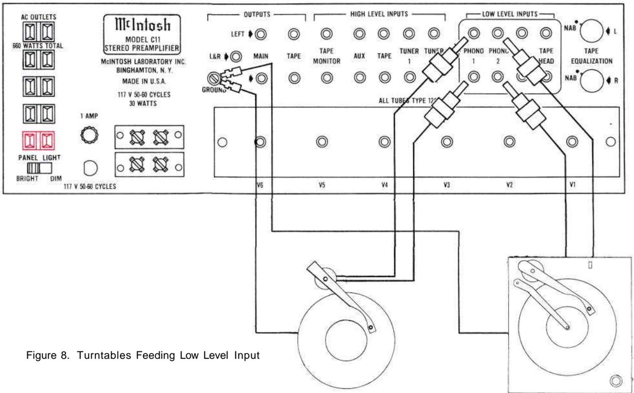
Figure 8. Turntables Feeding Low Level Input
