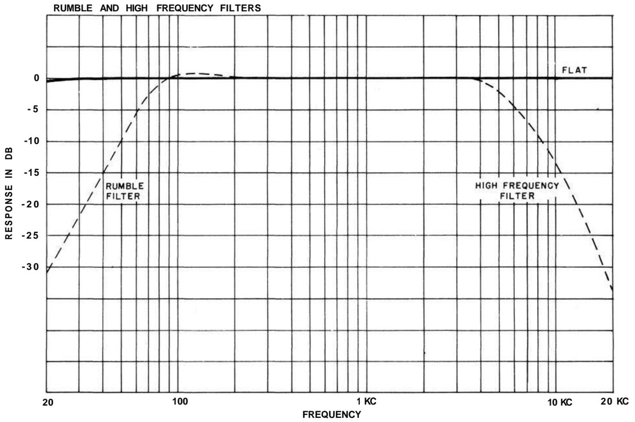
Figure 12. Rumble filter and high frequency filter.
