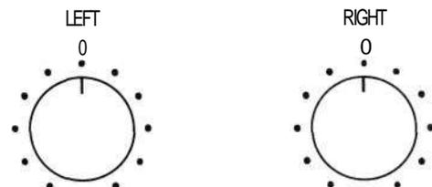
The LEFT and RIGHT TREBLE CONTROLS regulate treble loudness to the left and right speakers, respectively. Clockwise rotation increases treble loudness; counterclockwise rotation decreases treble loudness.
