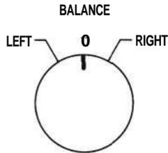
The C11 is balanced for unequal program sources by this control.
