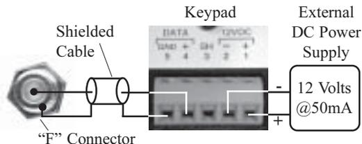
6. The WK 3/WK 4 Keypads are designed to be connected with a "four conductor shielded cable" or "CAT 5 shielded cable". In most installations a non shielded cable may be used with the WK 3/WK 4, however the shielded cable provides the best immunity from outside interference.
