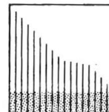
With Dolby replay the loudness of the previously amplified passages is lowered to normal; the frequency range is retained – the background hiss has disappeared.
