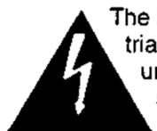
The lightning flash with arrowhead, within an equilateral triangle, is intended to alert the user of the presence of uninsulated "dangerous voltage" within the product's enclosure; that may be of sufficient magnitude to constitute a risk of electric shock to persons.
