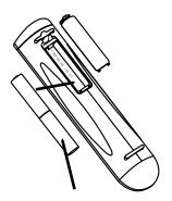
Press batteries into opening. Ensure correct fitting is observed.
