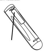
Press in and lift tab to remove battery cover out of recess.
