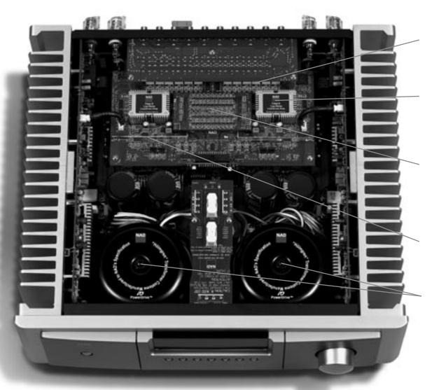
Sealed reed relay switches for superb signal integrity.
