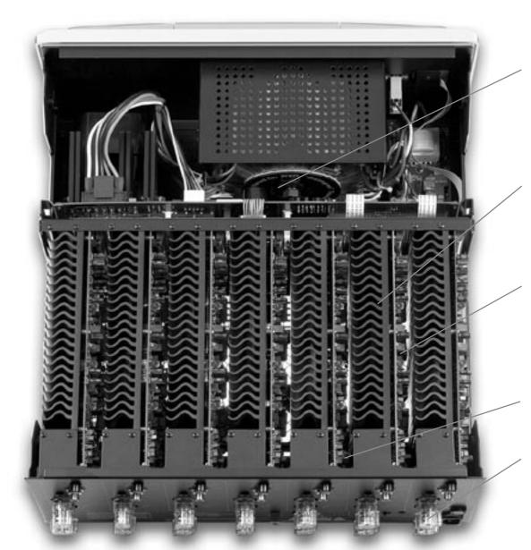
"Holmgren" custom-made transformers use special steel cores and winding techniques for excellent mains regulation and dynamic performance.
