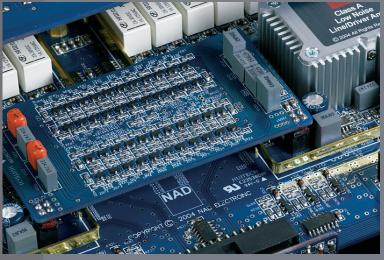
NAD's proprietary multi-stage discreet volume control circuit provides precise volume settings in 0.5dB increments with ultra high signal-to-noise ratio. Special NAD Class A gain modules provide tremendous dynamic headroom and nearly immeasurable distortion.
