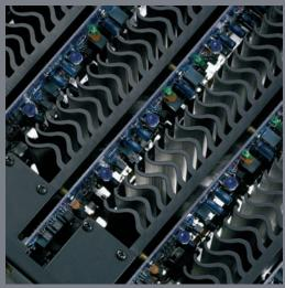
Unique NAD engineering. A 'wave form' heat sink fits 34% more cooling capacity into the same area as traditional designs. Greater thermal efficiency is aided by whisper fans that shut off during quiet passages.
