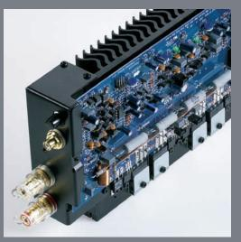
Each of the M25's seven channels is contained in a 'monoblock' gain module. So you benefit with the lowest distortion and widest channel separation. Effortless power adds emotional impact to your films.
