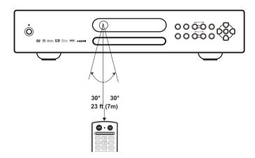
Distance: About 23 ft (7 m) from the front of the remote sensor Angle: About 30 degrees in each direction of the front of the remote sensor
