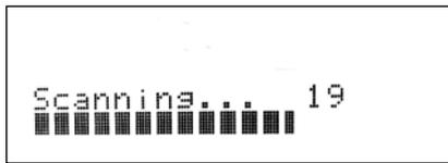
The bars show the progress of the sequence. When scanning is completed, the last number shown on the right side of the VFD corresponds to the total number of DAB broadcast stations found. Then, the first station is tuned in (See "ALPHANUMERIC" section below to understand the order or arrangement of stations).
