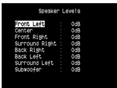
To produce the same SPL meter reading (or subjective loudness), use the remote's [▲/▼] keys to adjust each speaker.
