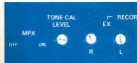
4 If away from 0dB, adjust the Tone Cal Level to obtain the accurate 0dB.
