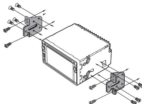
You may be able to install this unit in some makes of car without the supplied bracket.
