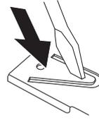
Bend the appropriate tabs to hold the sleeve firmly in place.
