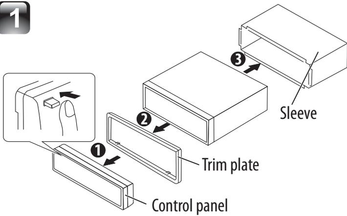
Bend the appropriate tabs to hold the sleeve firmly in place.
