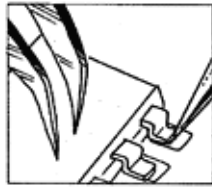
Secure the IC and solder.
