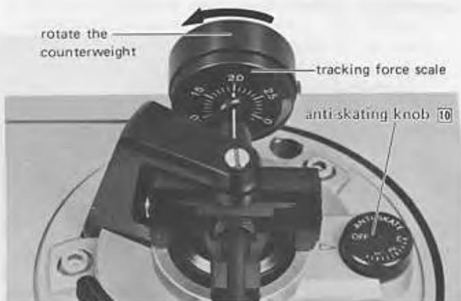
After setting the appropriate amount of tracking force, set the anti-skating knob **10** to the same value. If this is forgotten, the stylus may skid over the surface of the record during record play.
