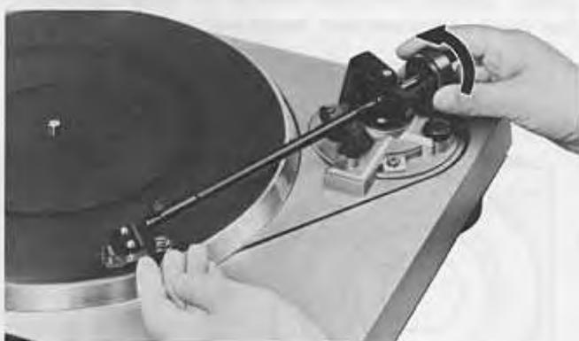
With the tonearm in this position, align the "0" on the scale ring **9** with the reference line on the tonearm by rotating the scale ring **9**. Note that the scale ring rotates along with the counterweight but the counterweight does not rotate when the scale ring alone is rotated.
