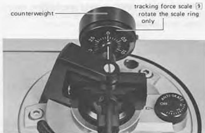
Now, slowly rotate the counterweight **8** in the direction of the arrow (the scale ring will also rotate) until the correct amount of tracking force for the cartridge in use is applied.
