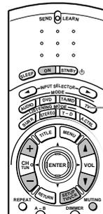
Press MODE TV first, then press the programmed TV operation buttons.
