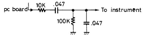
**Fig-35 B . P . F**
