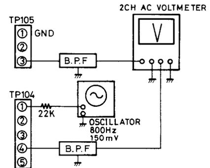
**Fig-38****4. Focus offset adjustment**
