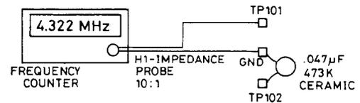
**Fig-36****2. Focus balance adjustment**
