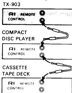
An **RI** remote control cable equipped with a 1/8" (3.5mm) diameter miniature two-conductor phone plug is attached to the TX-903 and to any compact disc player, with the **RI** mark.
