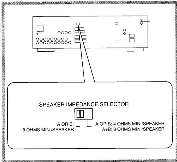
According to the impedance of the speakers used, set the SPEAKER INPEDANCE SELECTOR on the rear panel as shown in the table.
