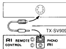
For this special cable Contact an ONKYO Service Center For a turntable (3.5mm pin to 7-pin plug cable) part number : 2010140
