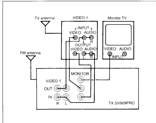
– If the television has no video input terminal, make the connections as shown below:–
