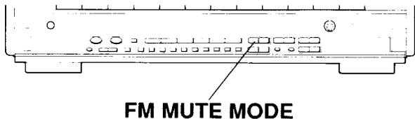
In the Muting ON (STEREO) setting, FM stereo reception is possible and the muting circuit suppresses interstation noise and weak FM stations. In the OFF (MONO) setting, interstation noise will be heard and even weak FM stations can be received. (Muting/mode operation is effective for only FM reception.)
