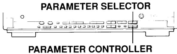
1. Press the ◀ or ▶ button of the PARAMETER SELECTOR to select balance.
