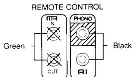
Connect a remote control cable to the black jack with the **RI** mark. Never connect it to the green jack with the **MTR** mark.
