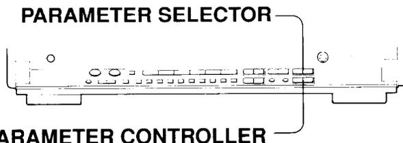
1. Use the ◀ or ▶ button of the parameter selector to select the parameter you want to adjust.
