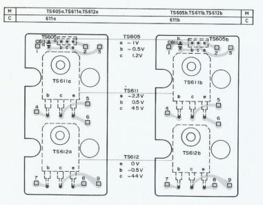
• TO BE MOUNTED 10mm A BOVE THE PRINT. • • TO BE MOUNTED 15mm A BOVE THE PRINT.
