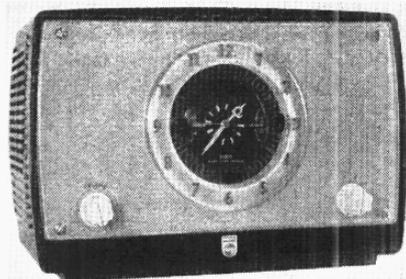
GIVING a choice of four pre-tuned stations, one on L.W. and three on M.W., the Philips 342A "Music Maid" also has a choice of several combinations of automatic switching operations which are performed by a synchronous type electric clock. Details of this latter feature are given overleaf under "Clock Operations."
