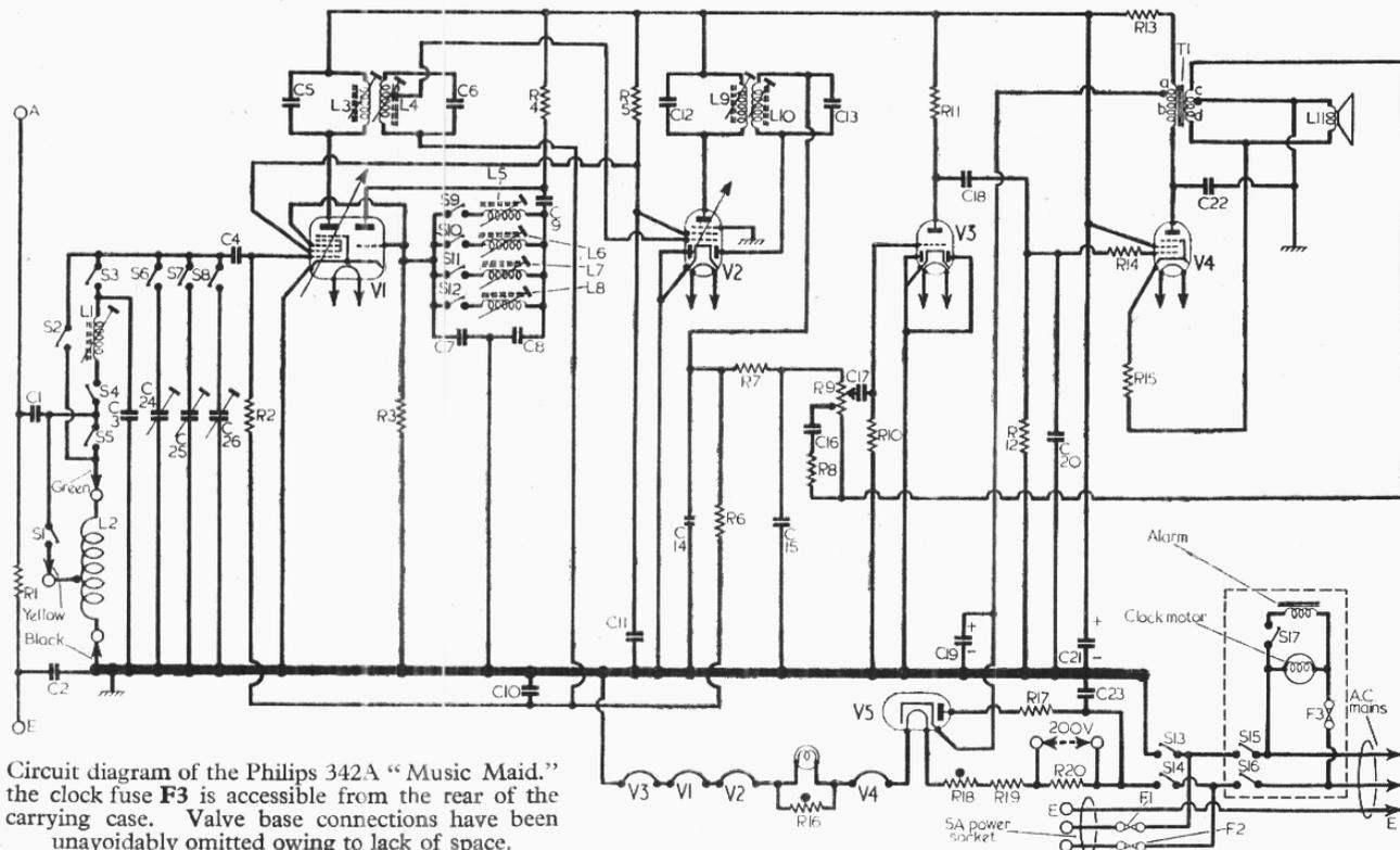
Circuit diagram of the Philips 342A "Music Maid." the clock fuse F3 is accessible from the rear of the carrying case. Valve base connections have been unavoidably omitted owing to lack of space.
