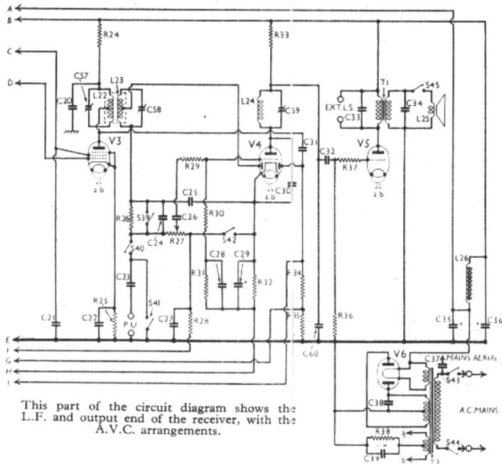
This part of the circuit diagram shows the L.F. and output end of the receiver, with the A.V.C. arrangements.
