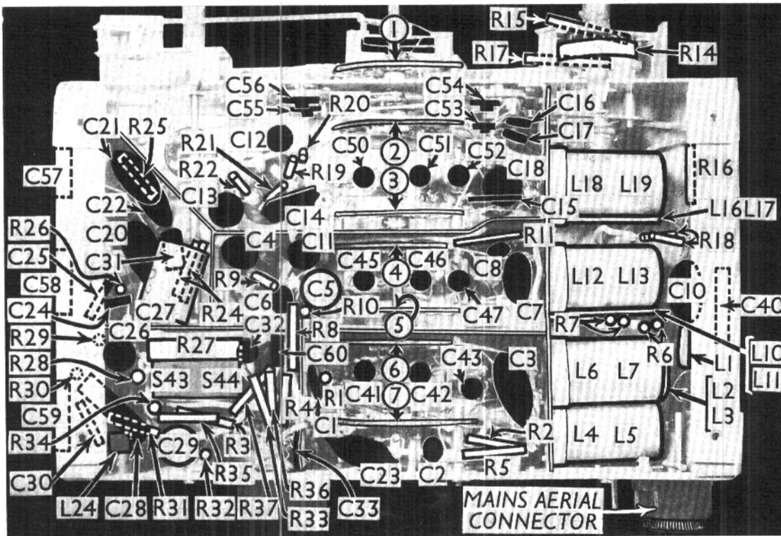
Under-chassis view. The switch units are numbered as in the diagrams above. **C53** is below **C54**, and **C55** below **C56**. **R25** is below **C21**. Some of the resistances consist of two units in parallel. Below the four coil units on the right are three further units, indicated by arrows. **R15** and **R17** are in front of the chassis.
