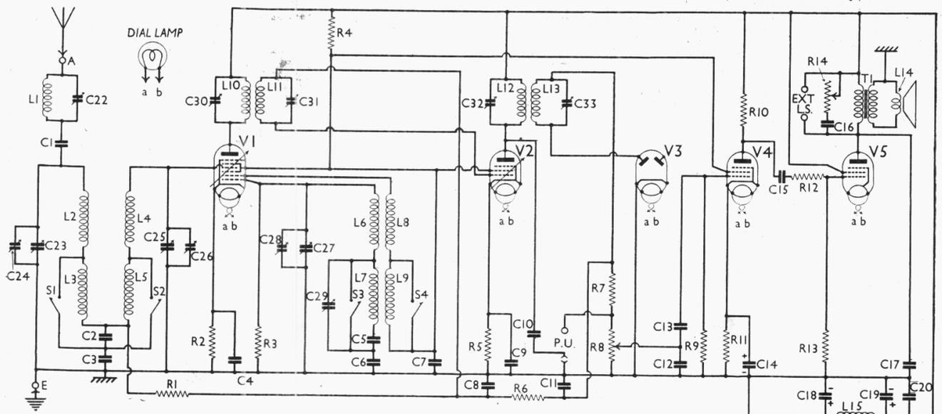
L.F. component is tapped off by manual volume control **R8** and passed on by way of coupling condenser **C13** to H.F. pentode L.F. amplifier (**V4, Mullard metallised SP4**). Provision for connection of gramophone pick-up across volume control. **C10** by-passes signals from **V2** when pick-up plugs are inserted.
