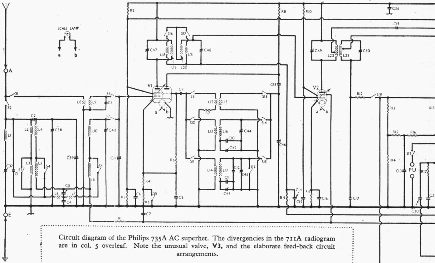
Circuit diagram of the Philips 735A AC superhet. The divergencies in the 711A radiogram are in col. 5 overleaf. Note the unusual valve, **V3**, and the elaborate feed-back circuit arrangements.
