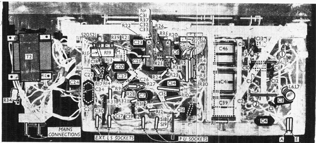
pentode section of V4. Fixed tone correction in anode circuit by C29. Variable tone control by C30, C34 and R22 between V4 anode and V3 cathode circuit. Provision for connection of low impedance external speaker across speaker secondary of output transformer T1.
