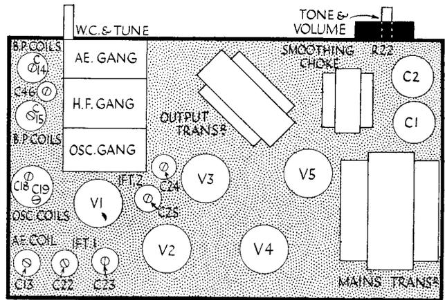
This drawing enables the components inside the Philips chassis to be identified. All resistors are indicated in solid black and condensers are shown in outline. This speeds reference to the diagram.
