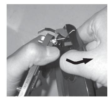
4.Bend the CD-door rightwards downwards as indicated in the picture above
