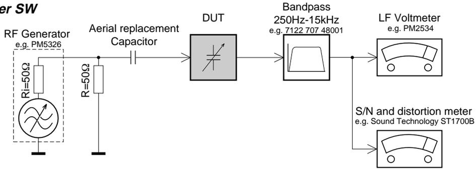
To avoid atmospheric interference all AM-measurements have to be carried out in a Faraday«s cage. Use a bandpass filter (or at least a high pass filter with 250Hz) to eliminate hum (50Hz, 100Hz).
