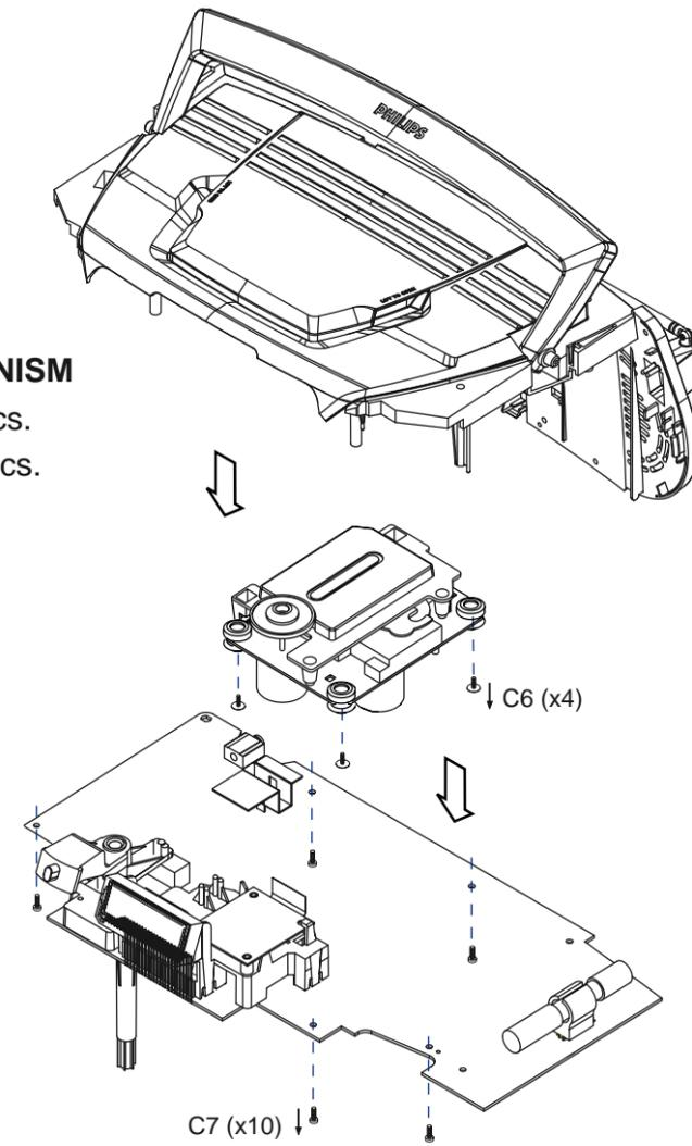
**D. TO REMOVE FRONT PANEL ASSEMBLY**
