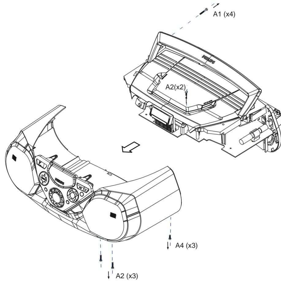
**B. TO REMOVE BATTERY COMPARTMENT ASSEMBLY**
