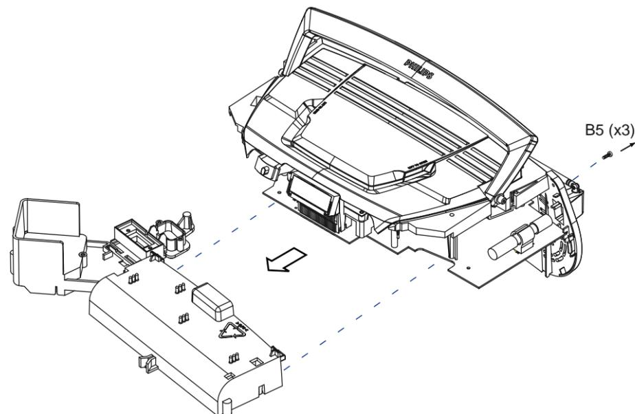
**C. TO REMOVE DECK MECHANISM**
